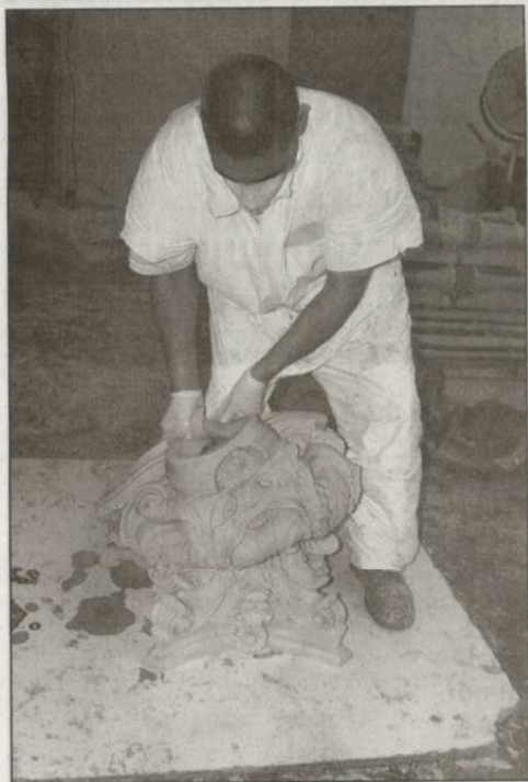
Left, Torres removes the mold from an already hardened capital. When completely cured, the capital can be used as a structural element, and will support more than 15,000 pounds when placed on top of a column.
